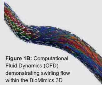
Figure 1B: Computational Fluid Dynamics (CFD) demonstrating swirling flow within the BioMimics 3D stent.
